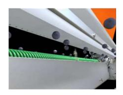
Tolaini's new **Optical Selection machine** uses state-of-the-art camera and light technology to analyze each berry for the perfect size, color and form. Any berries that do not meet the criteria (or foreign matter like bits of stem or bugs) are discarded by a jet of air. Only the best whole grapes make it into the vats to be made into wine.
